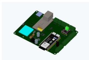
Controller, field IO and operator panel: renders from project STEP files
